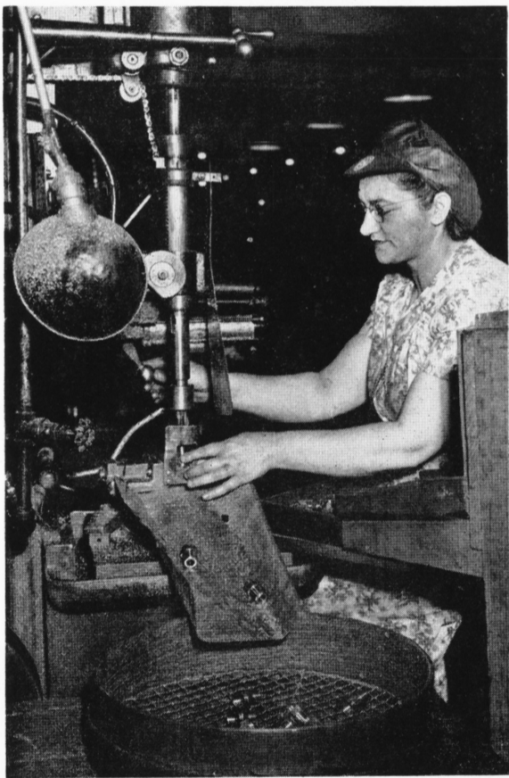
Following machining, the fittings-to-be move along to Chucking. Here, Susan Sacco performs the counterboring and tapping operations on the pipe end of a straight connector.
